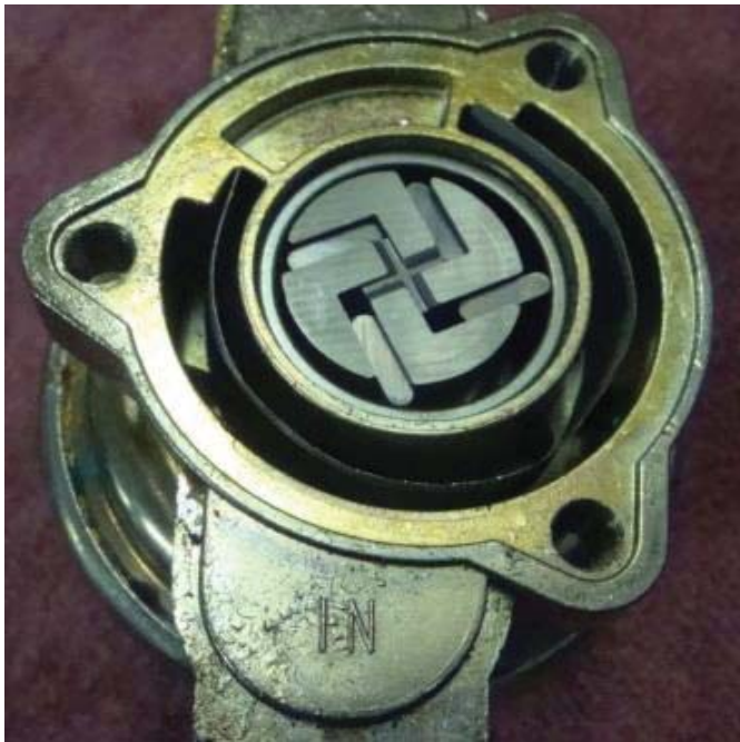
Carter P4259 6V rotary electric pump
