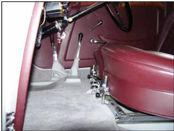
The position of the handbrake and in particular the shift lever make it all but impossible to use the driver's door for a graceful entry or exit. Notice, at the bottom of the front seats bracing that only an orthodontist could appreciate. This is the very unusual and avant-garde rake adjustment.
