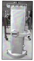
All main bearing caps and saddles were in fantastic shape. It was determined through using Plastigauge that clearances between the bearing surfaces and the crankshaft journals were well within Packard specifications.
