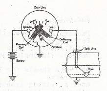
frame of the car. Turn on the ignition switch. The gauge should then read full. Remove the wire from the frame, with the ignition switch still on, and the gauge should read empty. If this is not the case, the dash unit should be replaced. If the gauge indicates as described, the trouble is probably in the tank unit, which should be replaced.
