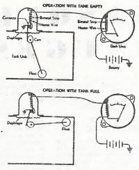
caused by the make and brake of the circuit is so small that the pointer seems to stand still. As the gasoline tank is filled, the cam on the float rod causes the contact to move to the right and therefore the strip in the tank unit must bend more before it breaks the circuit. This causes the strip in the dash unit to bend the same amount and moves the pointer toward the full mark on the dial. In this way the position of the float determines the position of the pointer in the dash unit.
